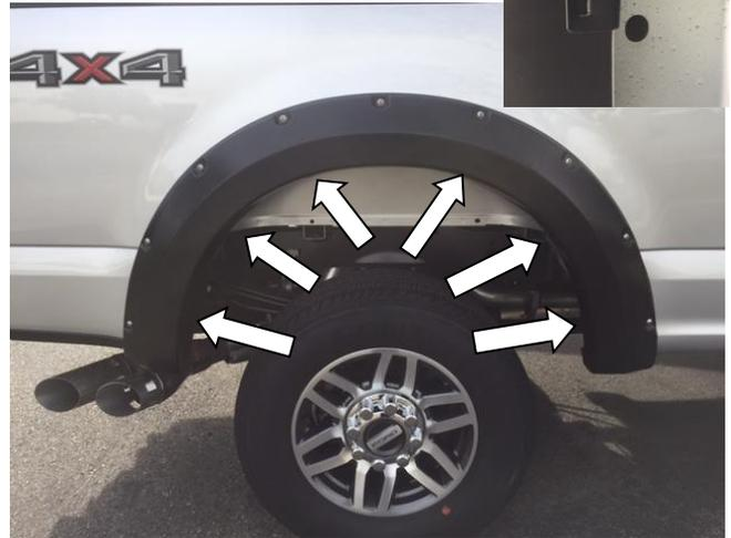
**STEP 11:** Place the Fender Flare onto the vehicle and fit into the correct position following the contours of the body. Use six (6) provided "U" Shaped Retention Clips to secure the Fender Flare to the body. Ensure the barb in the clip securely attaches in the slot on the Fender Flare. REPEAT ALL ABOVE STEPS FOR OPPOSITE SIDE OF VEHICLE.
