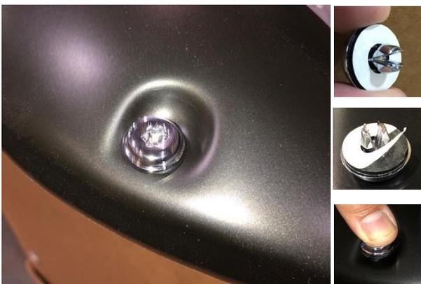
**STEP 8:** Attach the extruded plastic bolts. Peel back white tape liner from the bottom side of the extruded plastic bolt and press until it snaps into place. Ensure inside of Fender Flares where the rubber seal is attached is clean, using the alcohol wipes provided. Wipe away any residue with a dry clean cloth.
