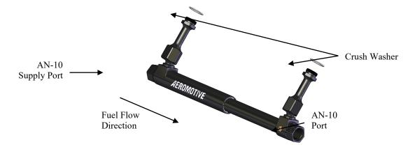
5. With the fuel log in place pivot the log to the position that provides the most clearance and tighten the pivot nuts to 20 in-lbs.
