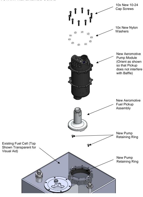
This product is intended to be installed and utilized for pump module replacement or upgrade of existing Aeromotive fuel pumps mounted on fuel cells which have already been plumbed and wired. If you are trying to install a pump module into a new cell or are replacing a non-Aeromotive pump, please contact the Aeromotive Tech Department for assistance with installation.
