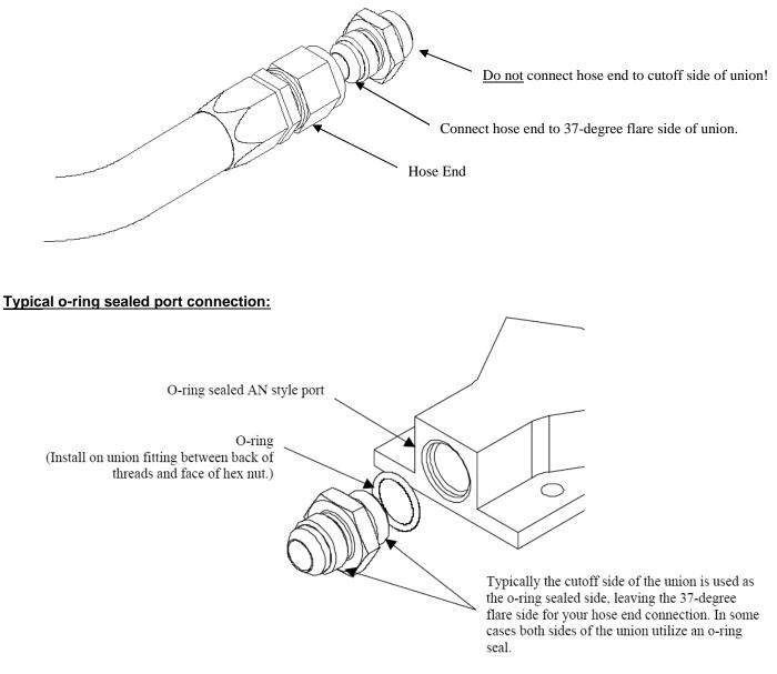
For example, in some systems an ORB to Flare fitting is used to connect the fuel pump and filter together, in which case you always install the ORB side into the fuel pump and the flare side with O-ring added into the filter.
