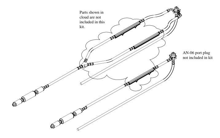
Note: Be sure to route all fuel lines clear of any moving suspension or drivetrain components and any exhaust components! Protect fuel lines from abrasion and road obstructions or debris.
