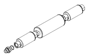
1-8. Install one of the supplied AN-10 o-rings on the AN-10 cutoff side of the AN-10 to AN-06 reducer union fitting, and install the fitting on the outlet side of the pump / filter assembly.
