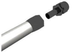
3-7. Using a properly sized wrench, complete threading the two components together (The maximum allowable gap between the two fitting components is .030 inches).
