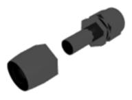
3-3. Insert hose in the socket with a twisting and pushing motion until the hose is fully seated in the socket.
