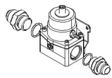
2-4. Install one of the supplied AN-06 o-rings on the cutoff side of the AN-06 cutoff union fitting and install in the AN-06 port located on the bottom of the supplied fuel pressure regulator.
