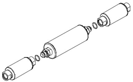
1-7. Install one of the supplied AN-10 o-rings on the cutoff side of the AN-10 to AN-08 reducer fitting and install on the inlet side of the pump / filter assembly.
