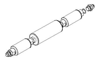
1-9. Find a suitable mounting location for the above pump / filter assembly. Typical mounting locations include mounting the fuel pump to the fuel tank shield or mounting to the inside of the frame rail. The fuel pump should be mounted as close to the fuel tank as possible and as low as possible. Using the fuel pump mounting clamps as a guide, mark the four pump mounting holes. Ensure there are no obstructions behind the mounting surface and drill four 1/4" mounting holes.
