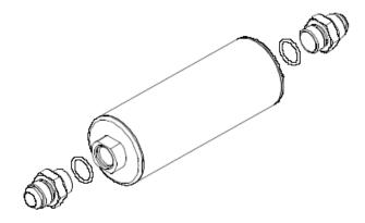
1-6. Noting the appropriate flow directions, install the provided fuel filter, Aeromotive p/n 12301, on the fuel pump outlet and the other fuel filter, Aeromotive p/n 12304, on the fuel pump inlet. If you get the two filters mixed-up, the 12304 filter will have a 100 micron stainless steel filter element inside, where as the 12301 will have a 10 micron paper filter element inside.
