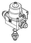
2-5. Starting from the fuel rails, plan a route to run an AN-06 feed line from each fuel rail to each side of the regulator. In the case of a single fuel rail system, only run one line from the fuel rail to the regulator. Cut the two supply line(s) to the determined length and install the AN-06 hose ends, as detailed in Section 3.
