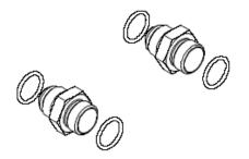
1-5. Install each of the two fittings into each end of the provided Aeromotive fuel pump.
