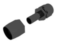
2-3. Insert hose in the socket with a twisting and pushing motion until the hose is fully seated in the socket.
