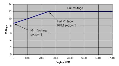
24. The initial pump voltage at idle or minimum voltage may also be adjusted by using a small screw driver and turning the "MIN VOLTS" screw on the front of the controller. Turning the adjustment screw counter-clockwise will decrease the initial pump voltage and clockwise will increase the initial pump voltage. This adjustment screw has a 15-turn range.
