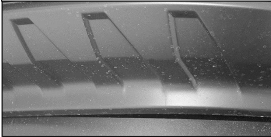
(Fig 4) Temporarily remove the splash guard as required to gain access to the front of the frame channel.
