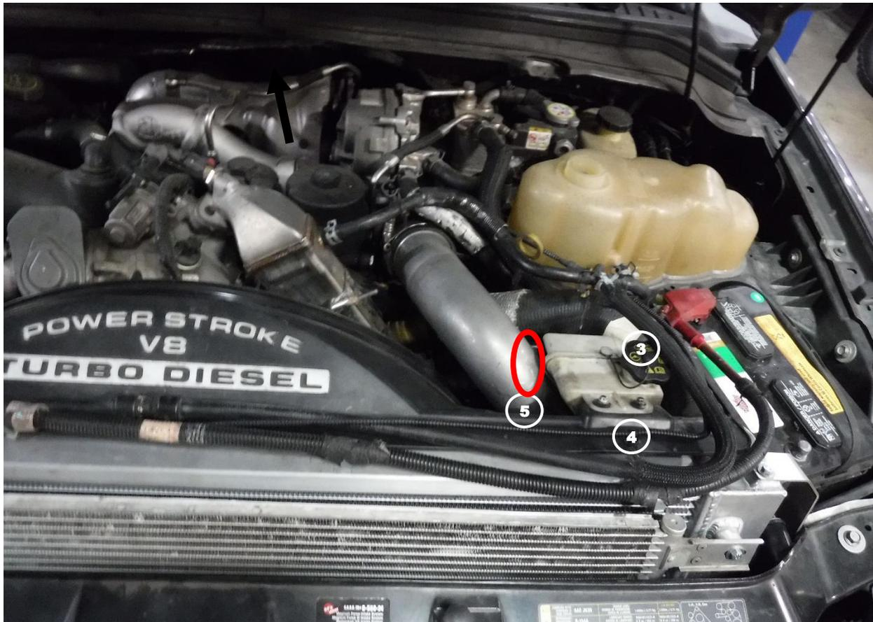
9. Unclip the power steering line from the power steering reservoir ③
