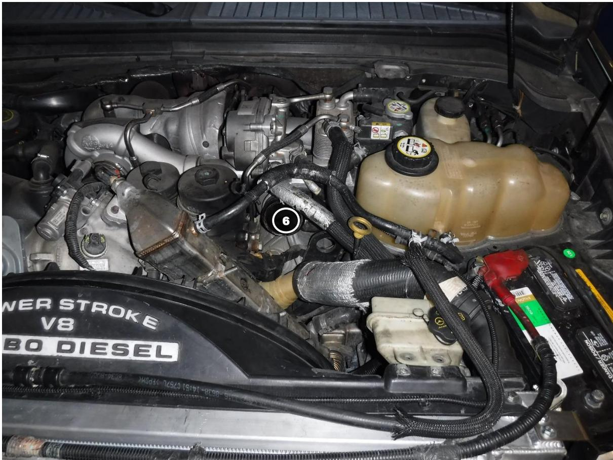
15. Loosen the clamp securing the turbo outlet coupling to the turbo ⑥ and remove the coupling and clamp from the vehicle.
