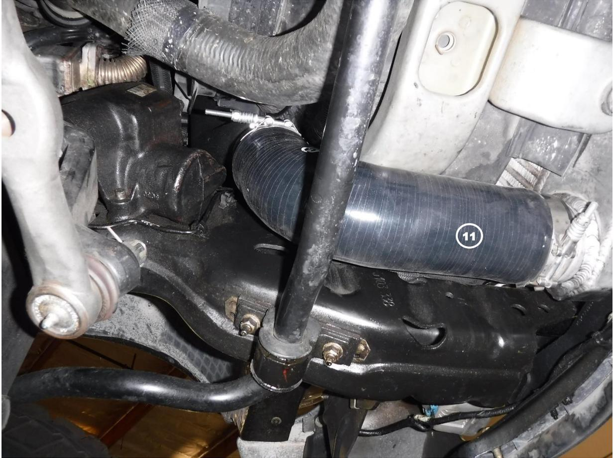
22. Install one (1) of the 3.25" spring-loaded T-Bolt clamps and the supplied 3.38" spring-loaded T-Bolt clamp onto the supplied aFe silicone reducing coupling, 3-1/4" x 3"ID 86 Deg, do not tighten the clamps yet.
