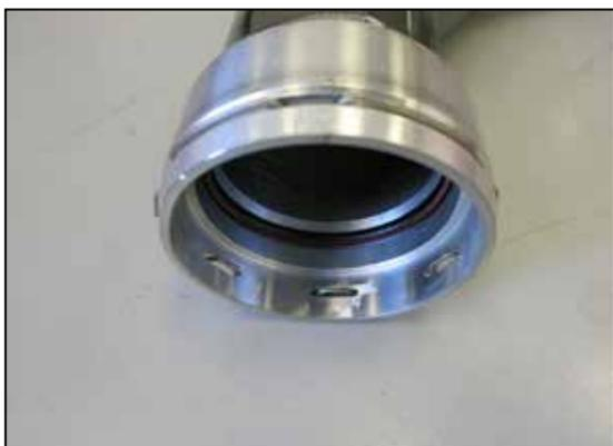
11. Remove the O-ring and retaining clip from the factory charge tube and install them into the K&N charge tube.
