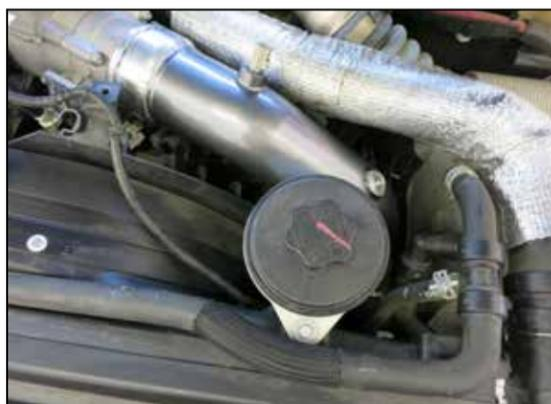
15. Reinstall the power steering reservoir and secure with the factory bolt.
