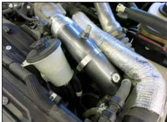
12. Install the K&N charge tube into the vehicle so the tube engages into the elbow coupler. **NOTE: Apply spray lube to the tube/elbow connection to aid the insertion of the tube into the coupler as it is a tight fit.**
