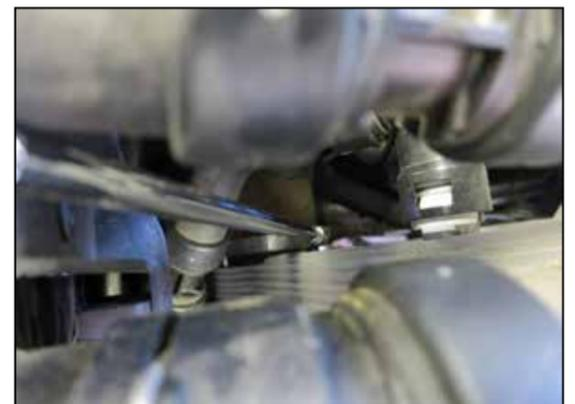
5. Using a 7mm socket, loosen the factory hose clamp that secures the charge tube to the inter cooler.
