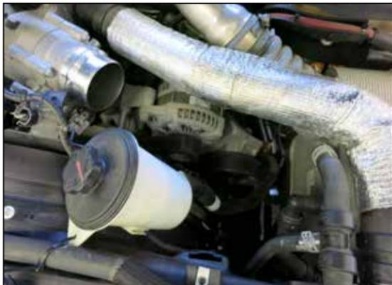
8. Remove the bolt that secures the power steering reservoir and set the reservoir to the side to aid with clearance during installation of the K&N charge tube.
