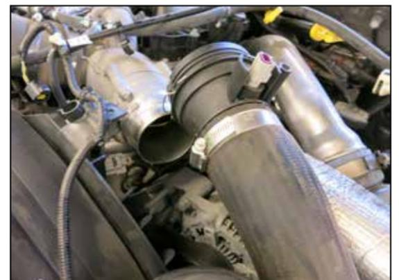
6. Separate the charge tube from the throttle body.
