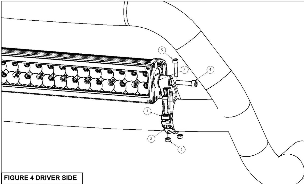
4. Mount the top and bottom clamps (items 1, 2, & 3) to the bar using (2) M6 socket head cap screws (item 5) and (2) M6 hex nuts (item 6) per clamp. **Figure 4** *Do not fully tighten at this time.*
