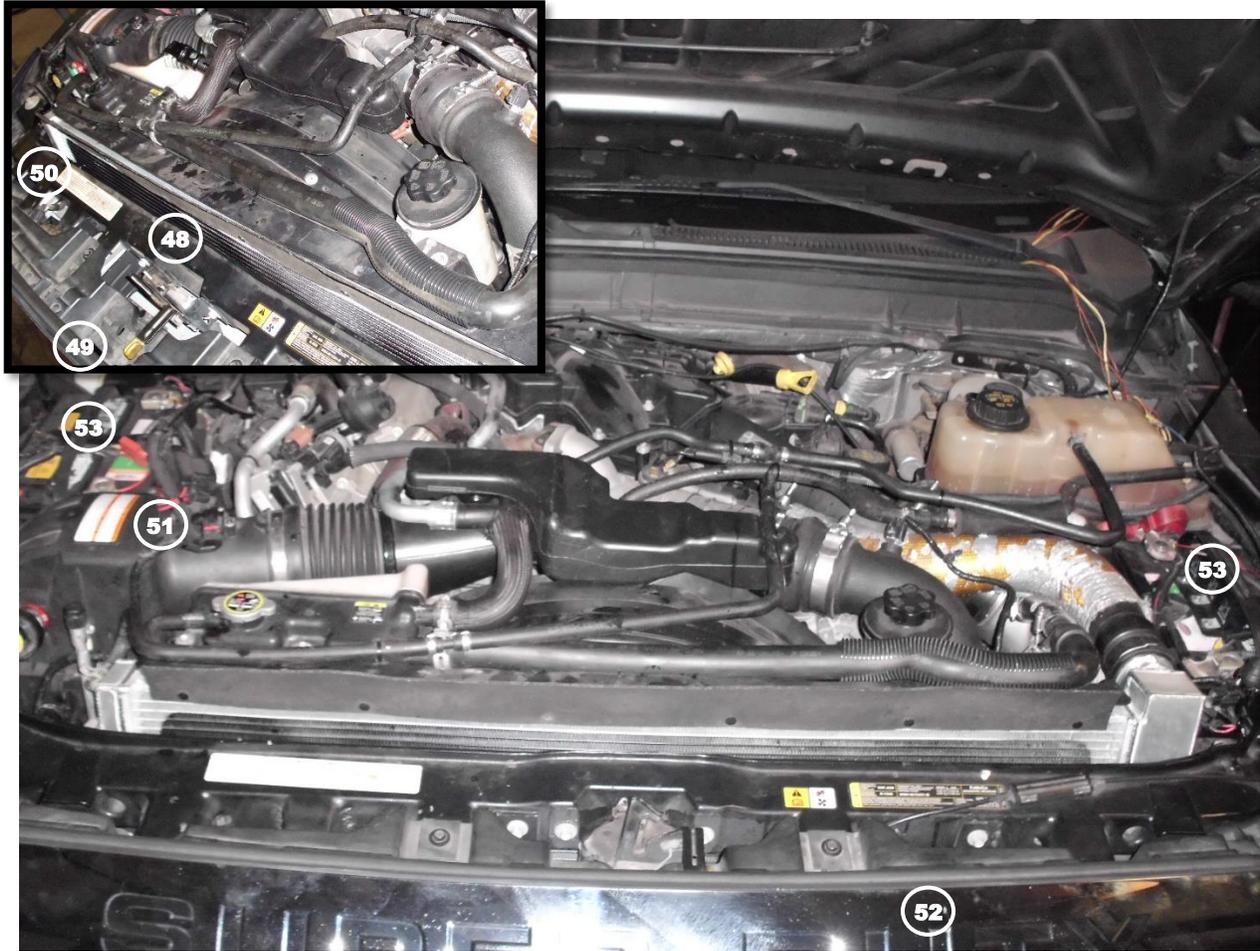
59. Reinstall the hood latch onto the core support (48) secure it using the factory hardware.
