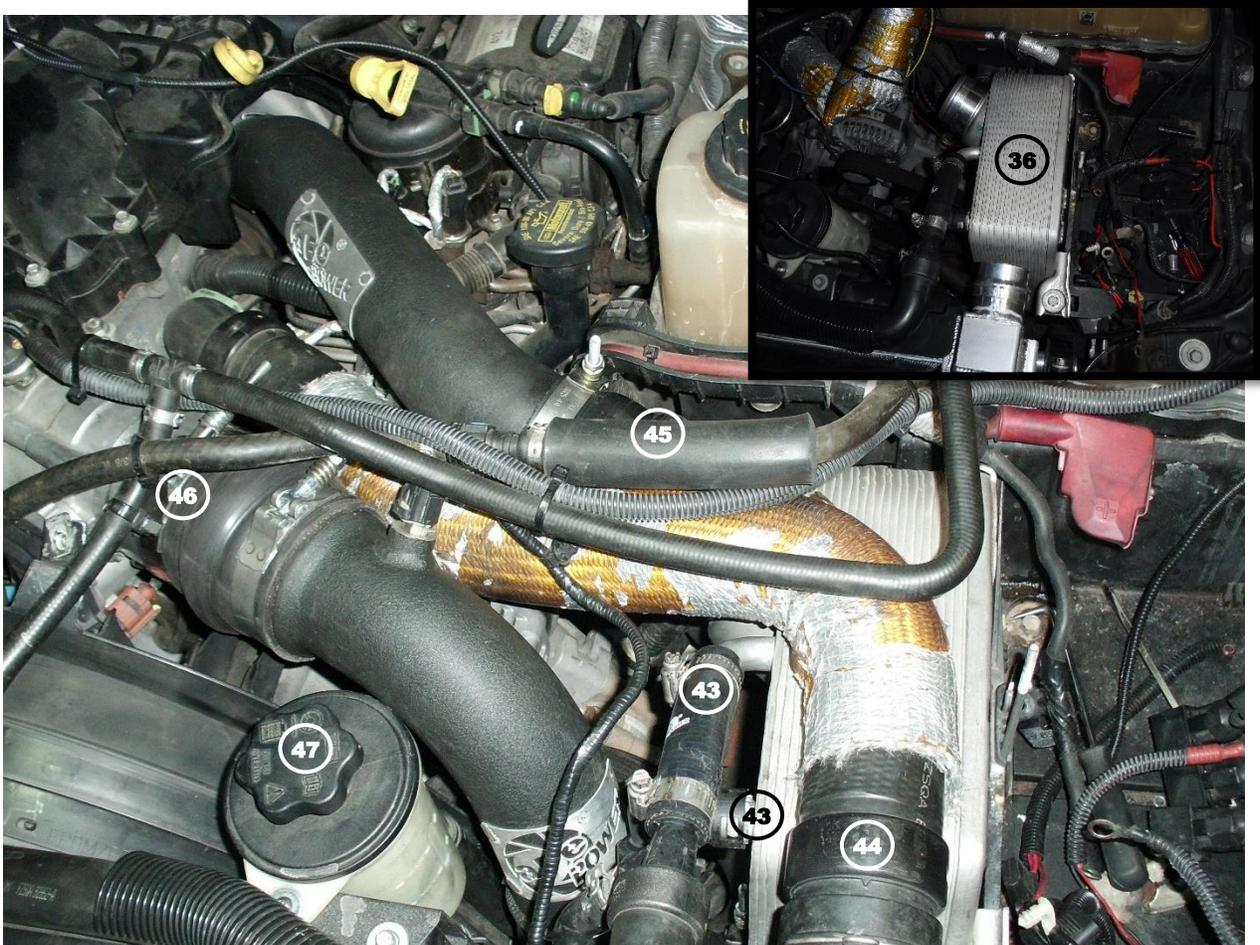
53. Reinstall the intercooler into the vehicle (42) secure it using the factory hardware.
