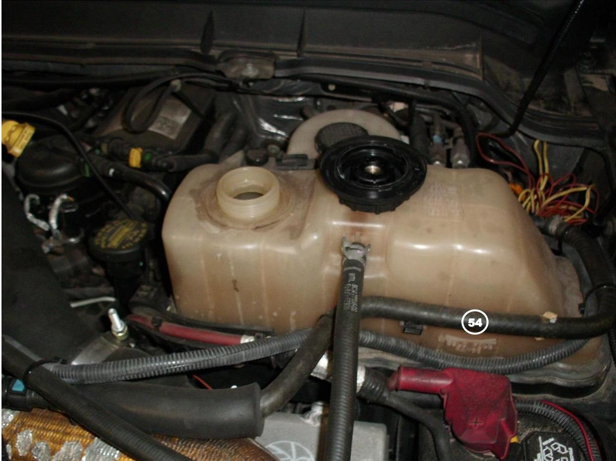
66. Use the proper coolant refill procedure to be sure that all the air gets out of the system when refilling the coolant for both reservoirs.
