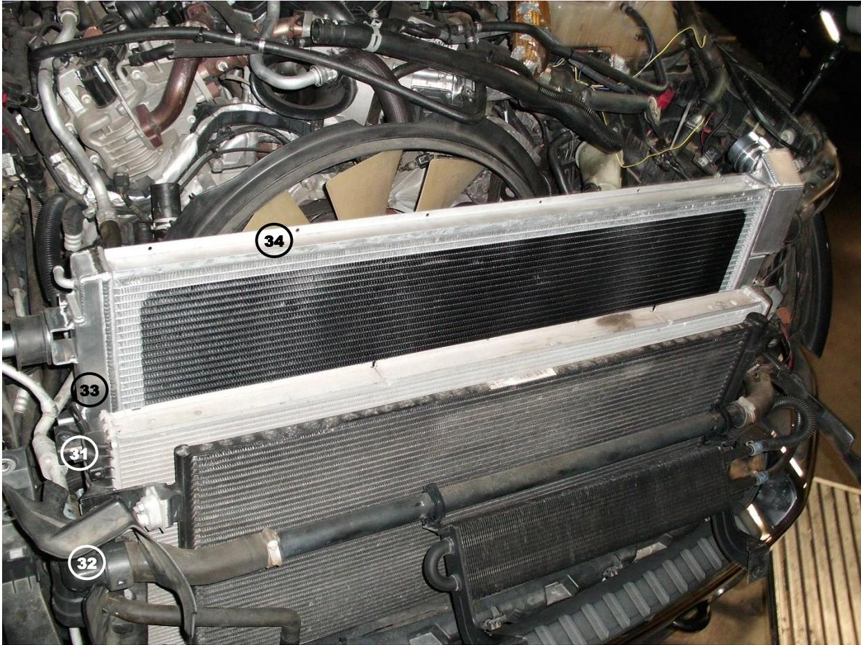
40. Install the aFe radiator onto the vehicle's lower mounting pins, ensuring the pins are positioned inside the grommets inside the radiator correctly.
