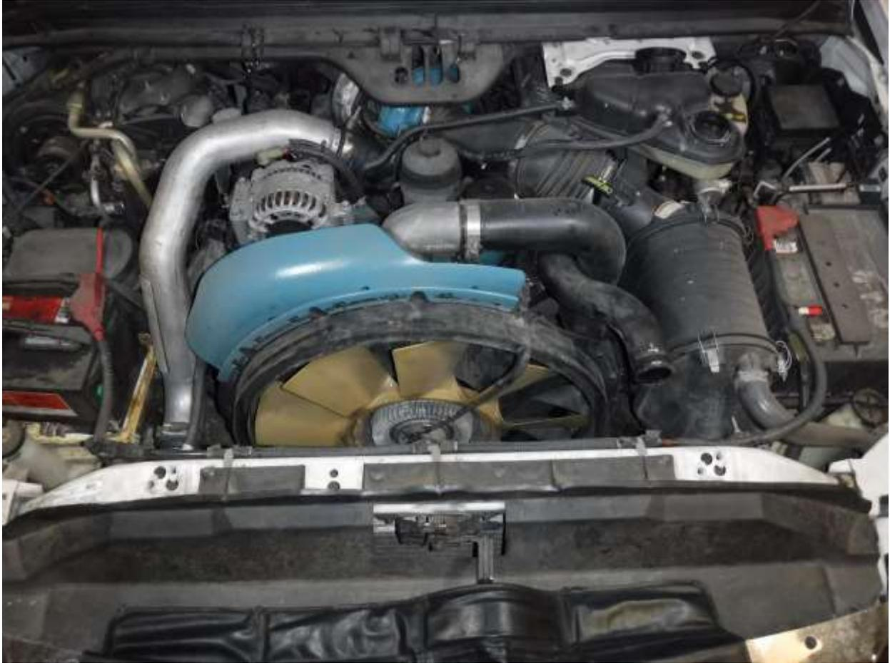
11. Remove the two (2) screws securing the fan shroud to the radiator.
