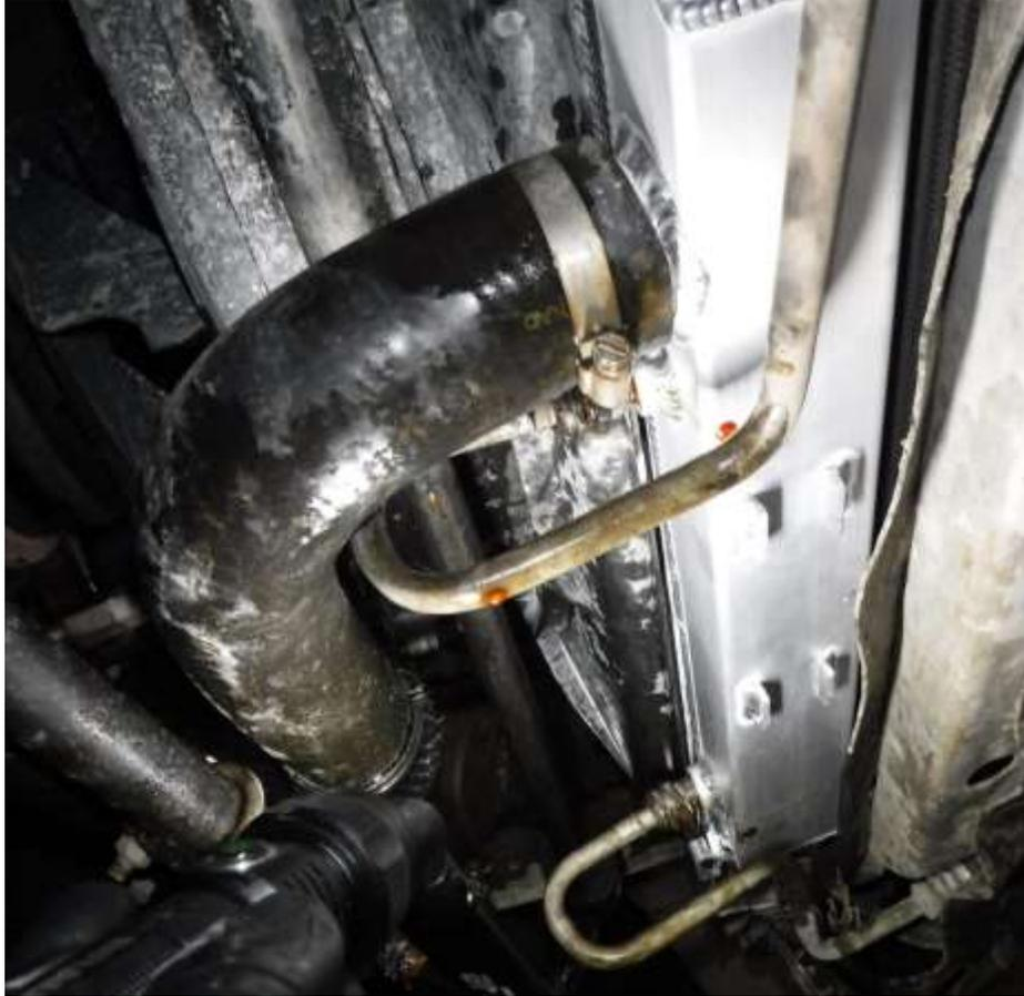
24. Secure the two (2) transmission cooler lines into the fittings on the aFe radiator. Be sure the retaining clip is properly clipped in all the way around (if equipped).
