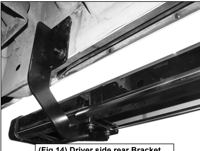
(Fig 14) Driver side rear Bracket attached to Running Board
