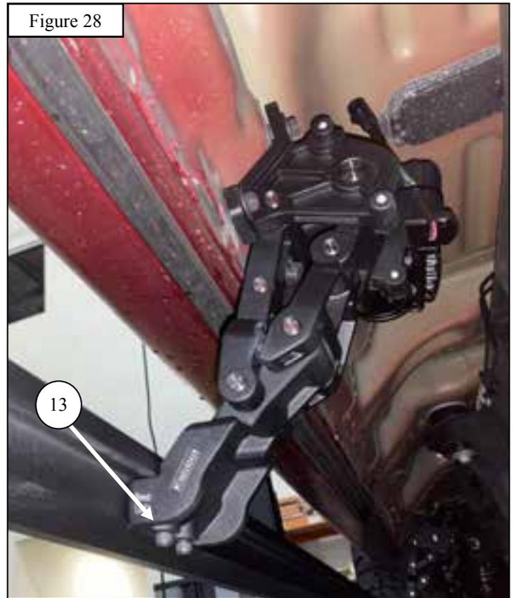
11. Locate and connect the previously routed male connectors from the main wiring harness to the female connectors on each motor linkage assembly. As mentioned previously, the male connector labeled “Front Left” will be connected to the female connector on the front driver side motor linkage, and the “Front Right” male connector should be connected to the female connector on the front passenger side motor linkage.
