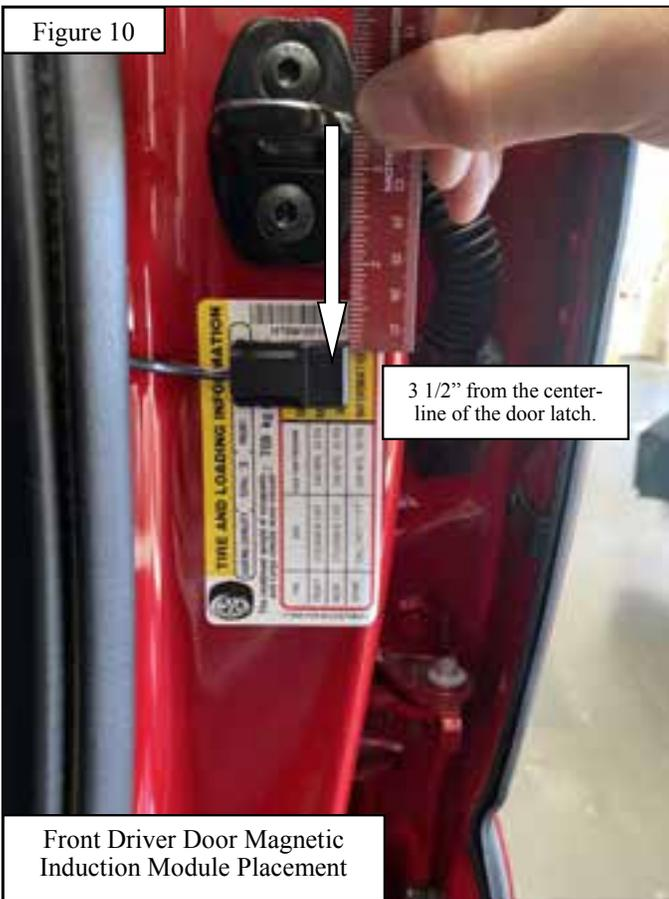
Front Driver Door Magnetic Induction Module Placement
