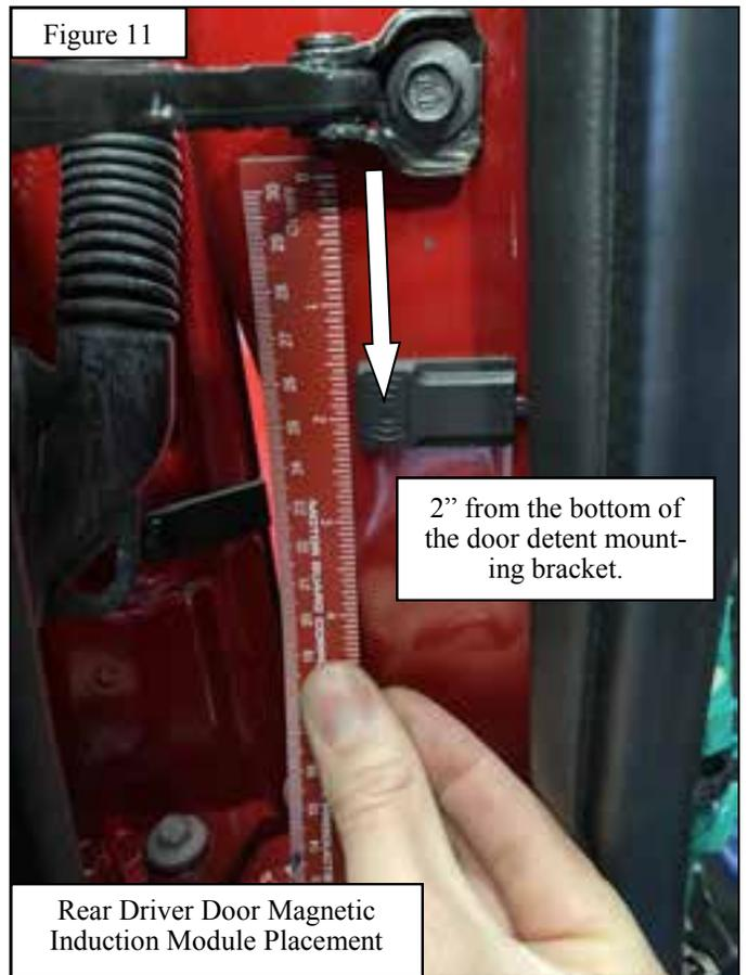
Rear Driver Door Magnetic Induction Module Placement
