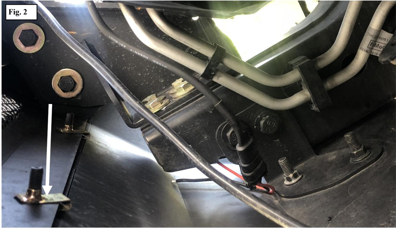
3. Instead of u-clip , use serrated flange M8 nut (Item 6) on the two bolts that attach to the side wings.
