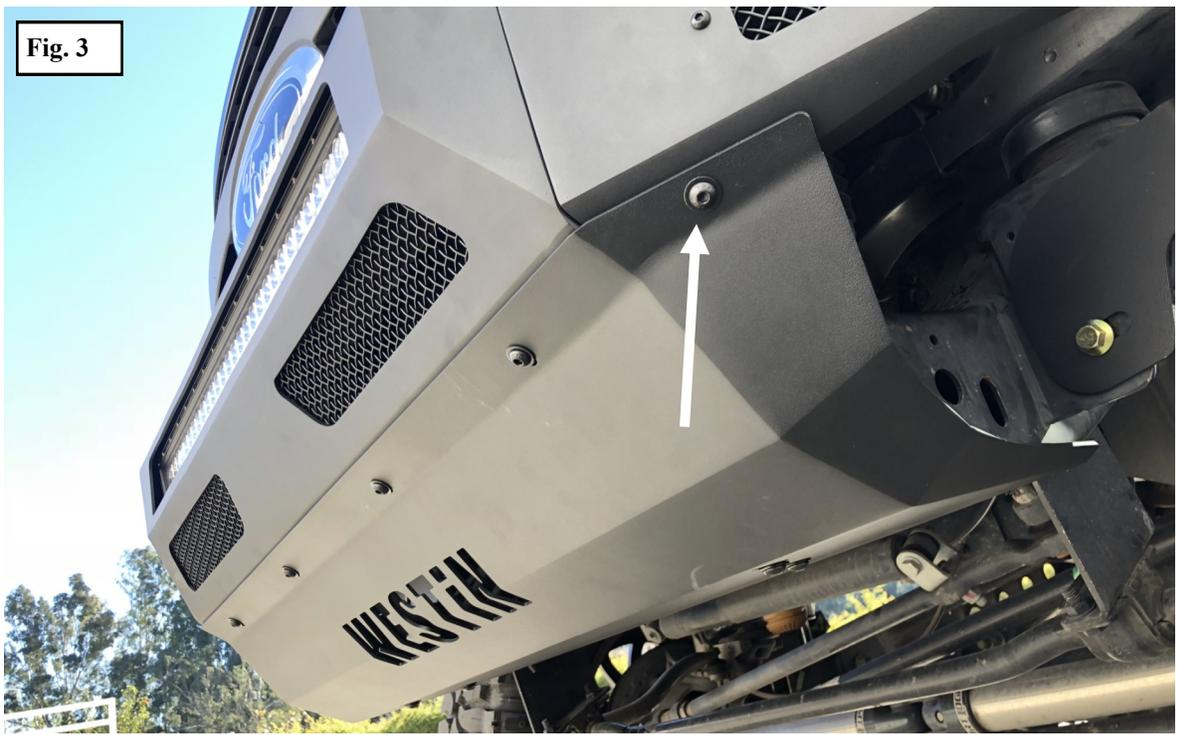
12. Align skid plate as desired and torque all hardware as specified: M8 to 18 ft-lbs, M10 to 38 ft-lbs, M12 to 60 ft-lbs.
