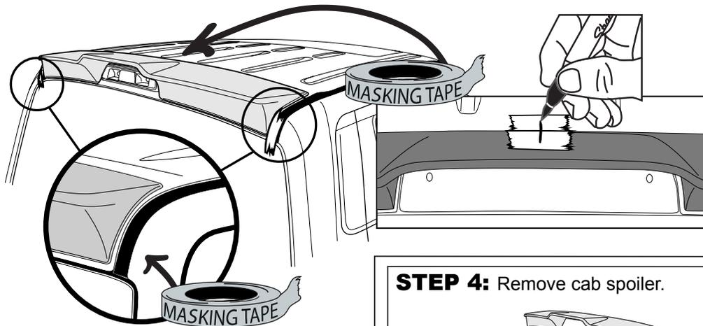
**STEP 3:** Place masking tape on roof aligning the edge of the masking tape to each end on the cab spoiler. Place masking tape centrally on the roof sheet metal and cab spoiler, mark line with a non-permanent pen to assist in positioning.
