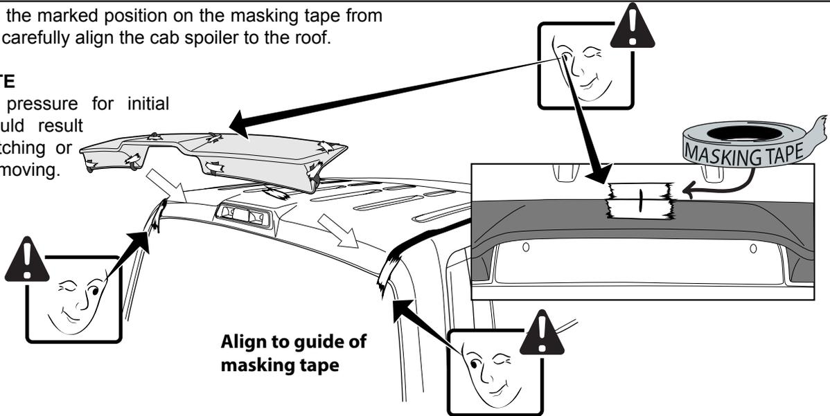
**STEP 8:** Once correctly positioned remove the tape liner from the cab spoiler.
