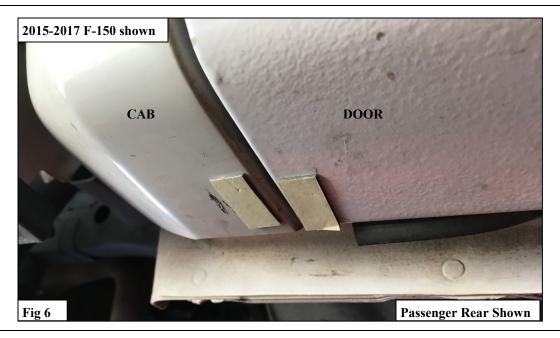
12. Place the magnetic switches on the double sided tape. *Note– it is extremely important that the switches face each other. They will not work if positioned incorrectly.* **See Figure 7.**
