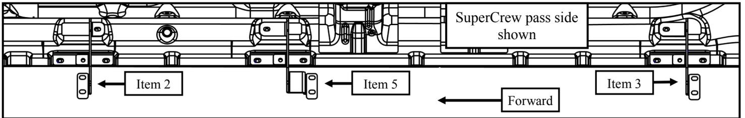
**NOTE :** (FOR SUPER CAB APPLICATIONS THE ORIENTATION OF BRACKETS ARE THE SAME. THE ONLY DIFFERENCE IS IT WILL **NOT** HAVE CENTER BRACKETS.)
