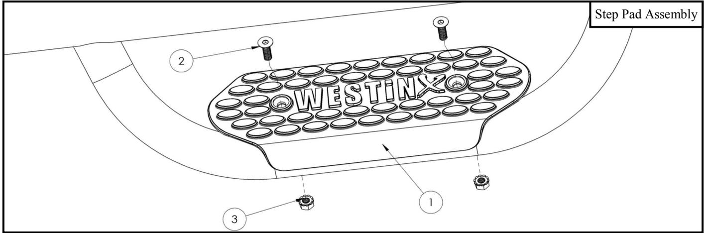
**ANTI-SEIZE LUBRICANT MUST BE USED ON ALL STAINLESS STEEL FASTENERS TO PREVENT THREAD DAMAGE AND GALLING .**
