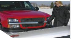
To begin plowing, remove pin, lift blade one end at a time and lower it over push frame, then replace the pin.
