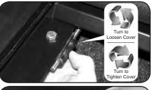
C. Check cover tension by releasing autolatch and open and close rear bar several times. It should snap down when closing. Cover fabric should sounds drumlike when tapped on. If adjustment is needed, roll cover open and turn EZ-Dial counter-clockwise to tighten, clockwise to loosen. Always turn dials in equal amounts.
