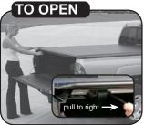
Open tailgate on driver side, pull autolatch and lift up on rear roll bar
