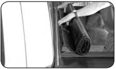
A. Set rolled up cover on rails at front of box (behind cab) with bar facing up. Roll cover bar onto front of rails and fold/tuck vinyl flap under. Now bar will face down. Let straps hang to inside of box.
