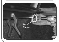
B. Hold rail in place with spring clamp and close tailgate to check height. Then place 1st clamp as close to front as possible and use ½" wrench to tighten.
