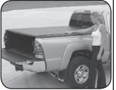
Now along side of box, seal cover edges with hook and loop sealing system the full length of cover on both sides. Pull with one hand - seal with other hand.
