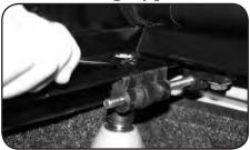
C. Hold bolt at top and tighten nut under side rail. Repeat procedure for right hand tension adjuster.
