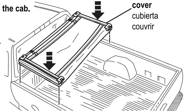
**Line up to front of bed first. Center the cover assembly on the truck.**
