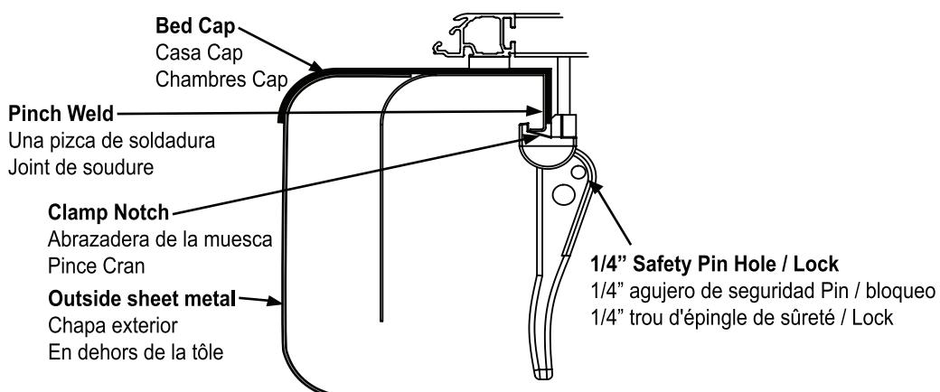
If traveling with the Tonneau in the folded position it is recommended to use a safety pin or lock in the front clamps.
