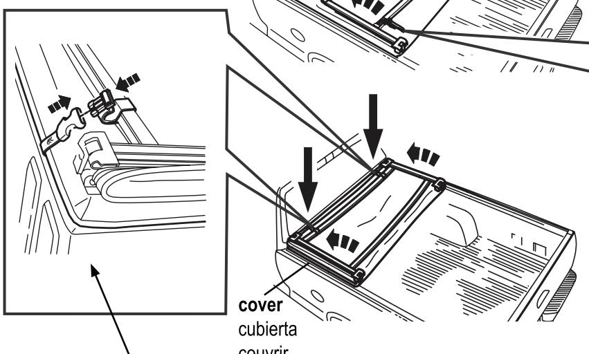
When stowing cover, position all clamps in their storage positions or latch handles may puncture cover and void warranty.
