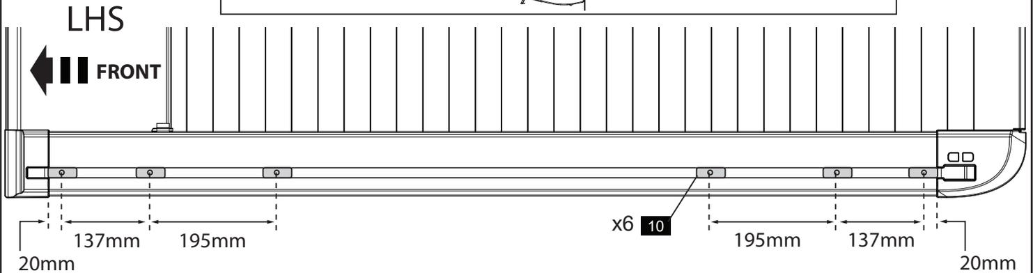
**1** Insert T-Nuts (10) into the LHS side rail T-channel. Position T-Nuts (10) in the T-channels using measurements as shown. Repeat for RHS.
