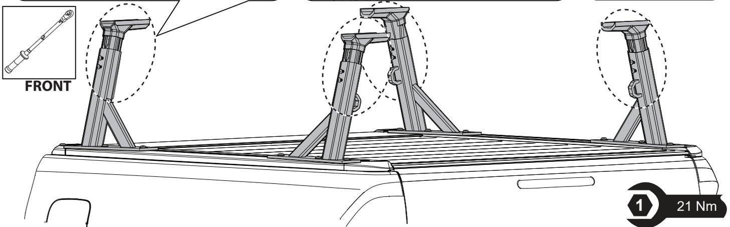
**3 IMPORTANT: DO NOT COMPLETELY REMOVE SCREWS UNLESS INSTRUCTED, ROTATE SCREW 2 TURNS MAX.**
