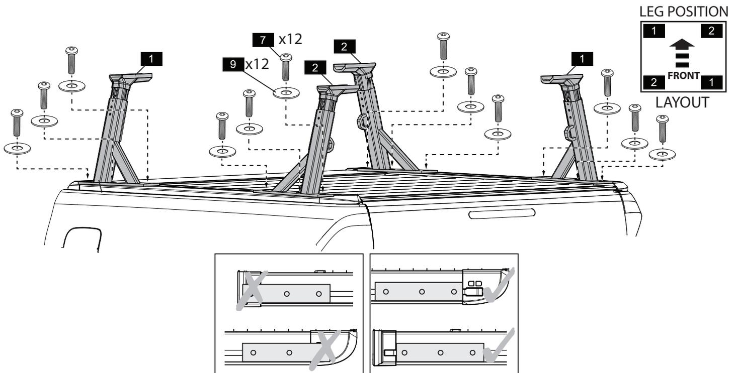
**2** Loosely attach legs (1,2) to the side rail extrusions using T Nuts (10) and M8x20 screws (7) and M8 Washers (9).
