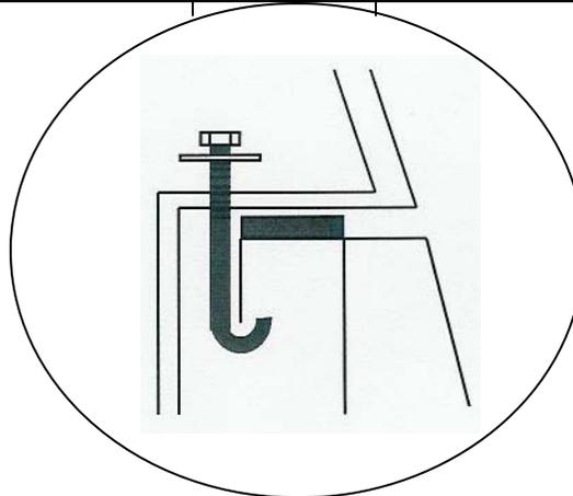
Step 1: Place foam tape (provided) under each end of the box that sits on the bed rail.
