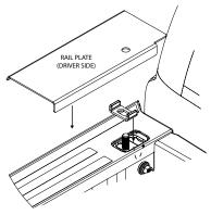
For the 30221 kit place rail plate over the stake pocket bolt and position notch against the front of the bed as shown
