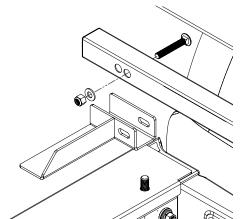
Fasten Backrack to the Rail mount bracket, or Toolbox bracket. Finger tighten at this stage.
