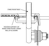
Cut away view showing support clip in correct position
