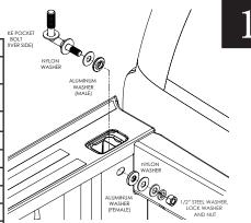
For each stake pocket bolt (driver and passenger) install nylon washer and aluminum washer over the rubberized end. Install the assembly into the stake pocket, and through the slot on the truck bed. Install the mating aluminum washer, nylon washer, 1/2" steel washer, lock washer and nut. Leave assembly finger tight at this stage.
