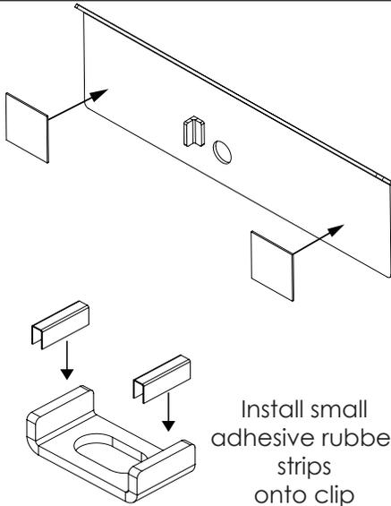
Install small adhesive rubber strips onto clip
