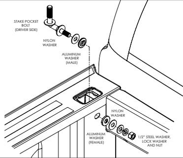
Fasten BACKRACK to the rail mount bracket. Finger tighten at this stage.
