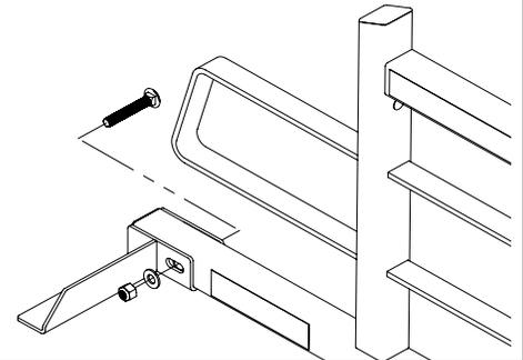
Fasten Backrack Assembly to the Stake pocket bolt as shown.
