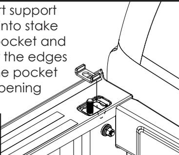
Cut away view showing support clip in correct position
